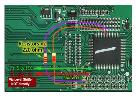
**NOTE:** It pays to use small dabs of hot-glue near the ATmega pins and in a couple of places along the wires to hold tl thing you want is for something to get hooked under them and rip them off, possibly damaging the ATmega pins in the
