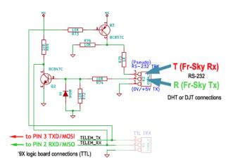
**NOTE** An earlier version of the above circuit had the collector and emitter of Q3 reversed. The circuit as shown here r circuit is clipped from the full schematic of the gruvin9x <u>custom controller board</u>.)
